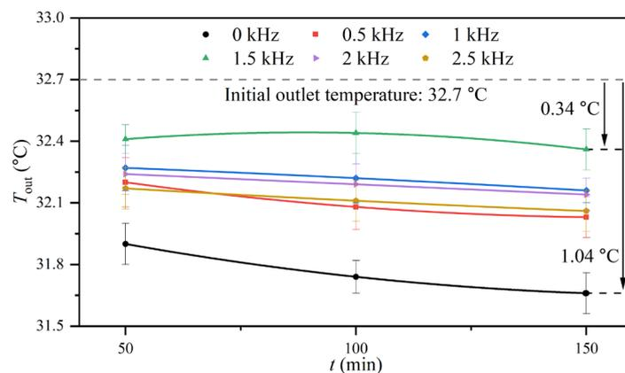
**Figure 9.** Outlet temperatures of experimental fluid at 50, 100, and 150 min under different electromagnetic frequencies.
