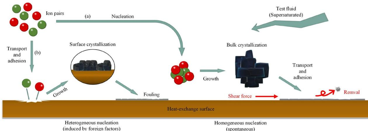
**Figure 3.** The formation process of crystallization fouling: (a): homogeneous precipitation; (b): heterogeneous precipitation.
