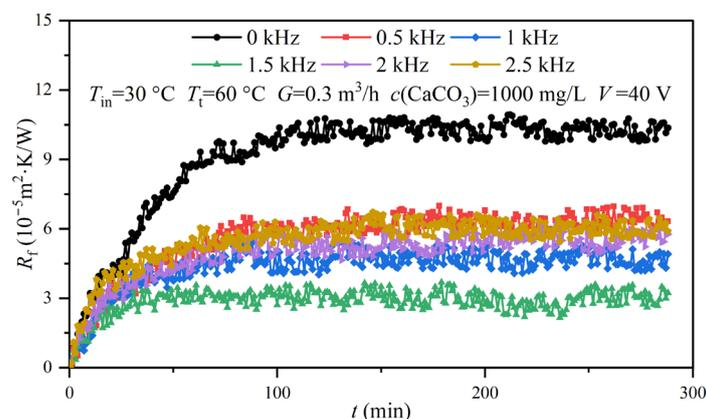
**Figure 5.** Fouling resistance curves under different electromagnetic frequencies.
