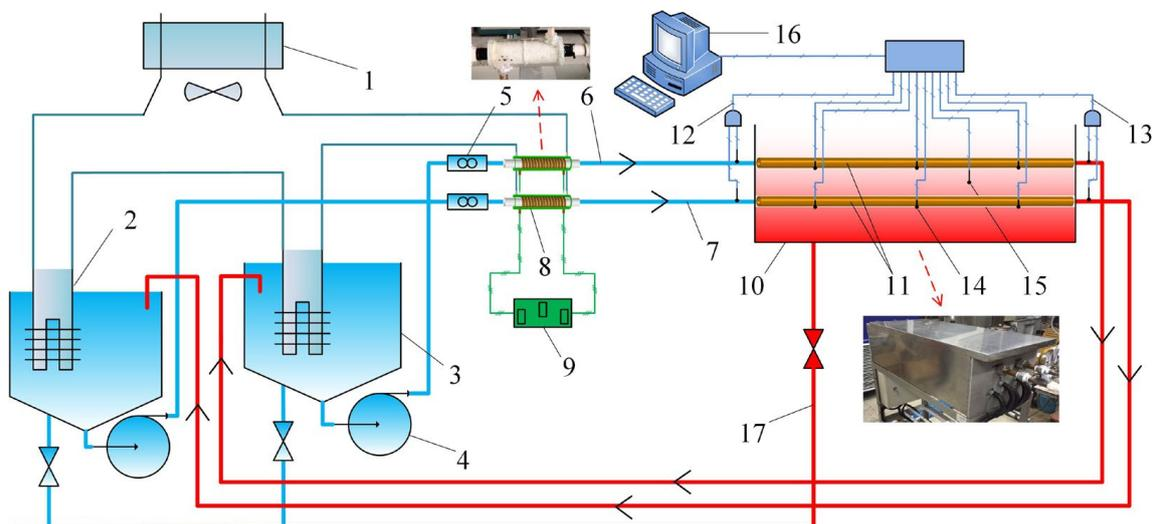
**Figure 1.** Schematic of the experimental rig. 1—Water chiller; 2—Cooling apparatus; 3—Experimental fluid tank; 4—Variable-frequency pump; 5—Ultrasonic flowmeter; 6—Circulation loop of side A; 7—Circulation loop of side B; 8—AEFTD; 9—Electromagnetic signal generator; 10—Thermostatic bath; 11—Shell-and-tube heat exchanger; 12—Inlet temperature; 13—Outlet temperature; 14—Wall temperature; 15—Bath temperature; 16—Data-acquisition system; 17—Drainage system.
