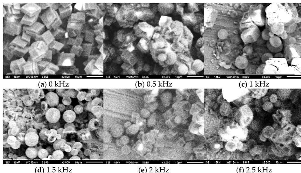
**Figure 10.** SEM micrographs of fouling samples under different electromagnetic frequencies.
