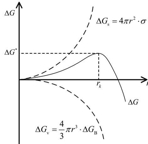
**Figure 11.** The relationship between the free energy variation and the radius of the crystal nucleus.
