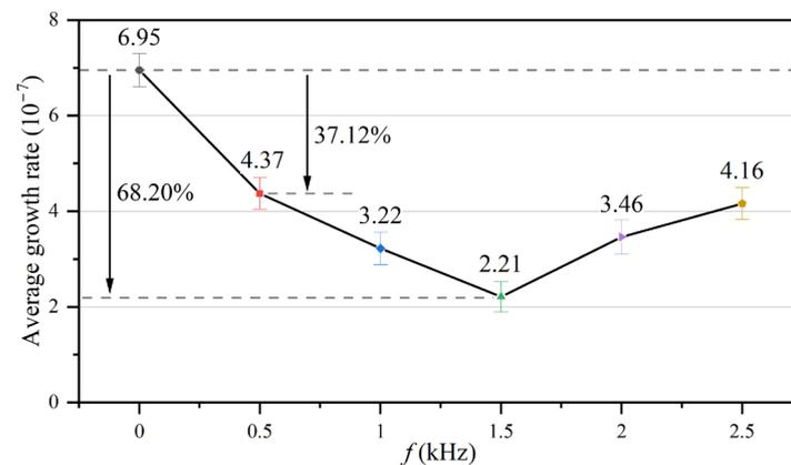
**Figure 8.** Average growth rates of  $\text{CaCO}_3$  fouling under different electromagnetic frequencies.
