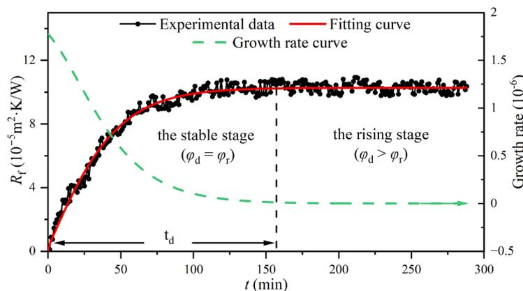
Figure 7. Fitting and growth rate curves of the fouling resistance in the control group.
