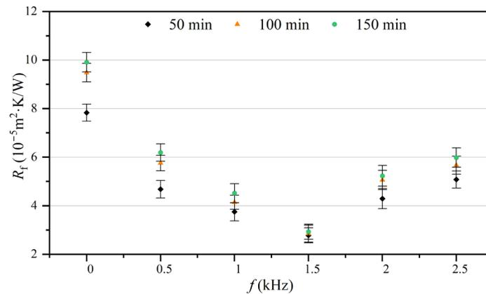
**Figure 6.** Fouling resistances at 50, 100, and 150 min under different electromagnetic frequencies.
