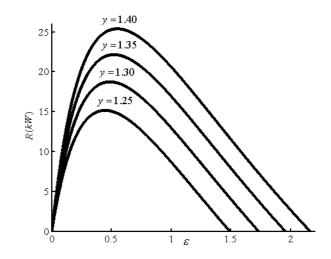
Fig.4 The influence of y on the optimal cooling load R versus the COP  $\varepsilon$
