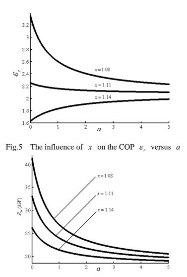
Fig.6 The influence of x on the maximum cooling load  $R_m$  versus a
