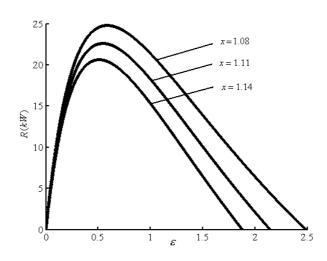
Fig.3 The influence of x on the optimal cooling load R versus the COP  $\varepsilon$
