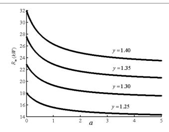
Fig.9 The influence of y on the maximum cooling load  $R_m$  versus a
