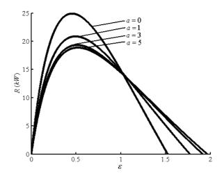
Fig.2 The influence of a on the optimal cooling load R versus the COP  $\varepsilon$
