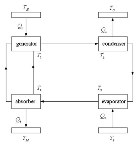
Fig.1 A four-heat-reservoir endoreversible absorption cycle model
