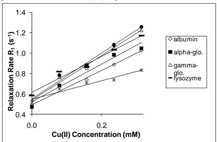
Figure 2. The Spin-lattice Relaxation rates (R<sub>1</sub>) of protein solutions versus concentration of Cu(II).
