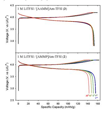
**Figure 3.** The charge–discharge voltage profiles of Li/1.0 M LiTFSI in ILs/LiCoO<sub>2</sub> cells.
