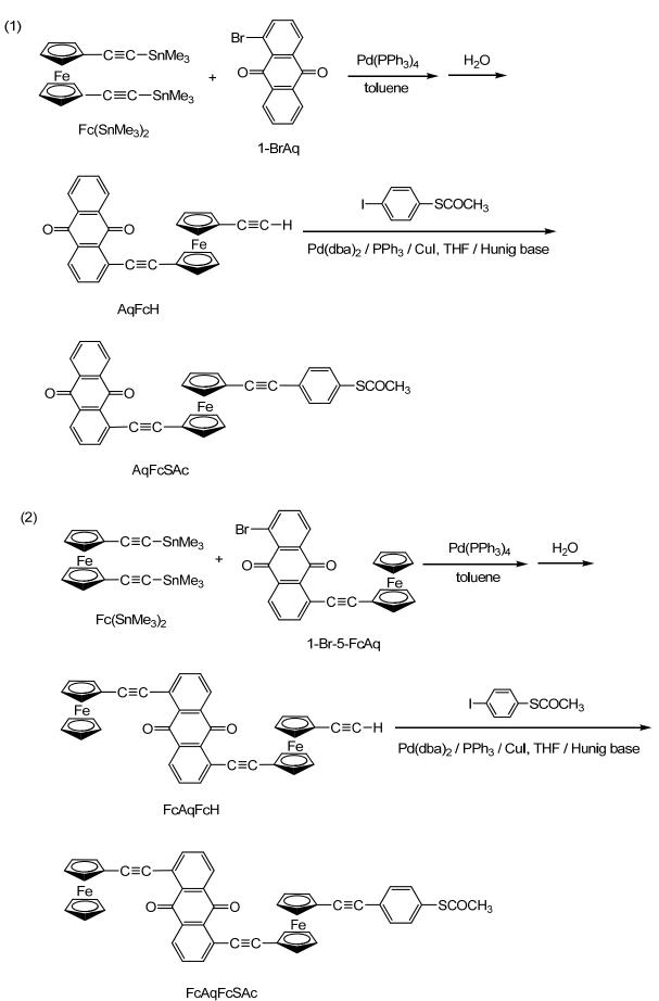
Scheme 2. The synthesis of AqFcSAc and FcAqFcSAc.
