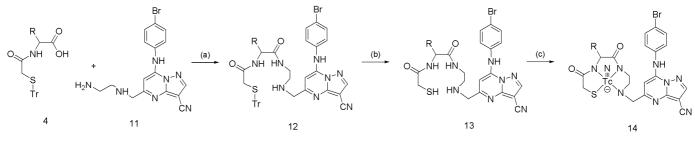
R=H, 4a, 12a, 13a, 14a; R=Benzyl, 4b, 12b, 13b, 14b; R=Isopropyl, 4c, 12c, 13c, 14c. (a) HOBt, DCC, Et<sub>3</sub>N, CH<sub>2</sub>Cl<sub>2</sub>; (b) Et<sub>3</sub>SiH, TFA; (c) <sup>99m</sup>Tc-SDH.
