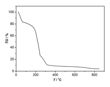
Figure 6. The TG-DTG curve of complex 1.
