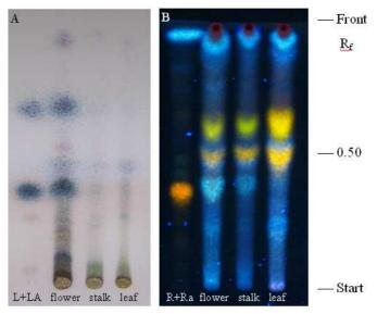
Experimental conditions: HPTLC silica gel 60  $F_{254}$  plate; (**A**) toluene:ethyl acetate 93:7 as mobile phase, vanillin-sulfuric acid for detection, 110 °C, Vis; L: linalool ( $R_f = 0.38$ ) and LA: linalyl acetate ( $R_f = 0.69$ ) as reference; (**B**) ethyl acetate:formic acid:water 8:1:1 as mobile phase, NST/PEG for detection, UV 365 nm; R: rutin ( $R_f = 0.36$ ) and Ra: rosmarinic acid ( $R_f = 0.94$ ) as reference.
