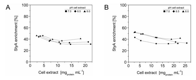
**Figure 3.** StyA immobilization efficiency from *Escherichia coli* JM101 (pSPZ10) cell extract on (A) Sepabeads EC-EA and (B) Sepabeads EC-Q1A at various pH values. Efficiencies are based on the ratios of adsorbed over soluble StyA at binding equilibrium.
