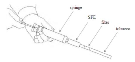
Figure 3. The installation for simulating human smoking.
