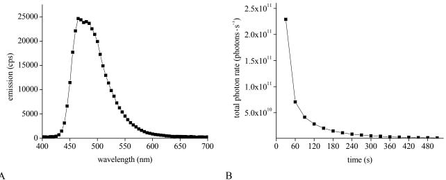
**Figure 8.** Spectral characteristics of LEDs: The spectral characteristics of the blue-emitting LED  $\lambda_{max} = 465$  nm and the green emitting LED  $\lambda_{max} = 525$  nm were recorded at the operating current of 18.5 mA (A). Operating current *versus* photon emission rate is displayed in (**B**).
