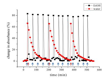
Our results, obtained with the application of several interconversion cycles between the spiropyran form and the merocyanine form, also clearly displayed that the amount of photobleaching is greatly reduced using low power LED illumination with  $1.754 \times 10^{16}$  photons s<sup>-1</sup> which has also been previously reported by Scarmagnani *et al.* [17].
