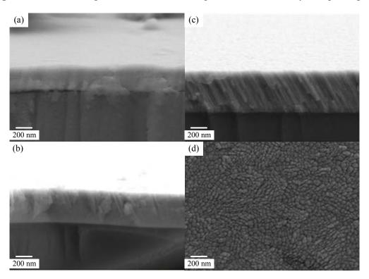
Figure 2. FESEM image of OAD-InN films deposited with variously oblique-angles.
