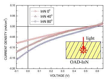
**Figure 7.** The J-V characteristics of the solar cells with OAD-InN sputtered at various oblique angles. The inset shows the light incident into the OAD-InN film.
