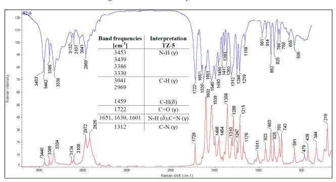
Figure 3. IR and Raman spectra of TZ-5.
