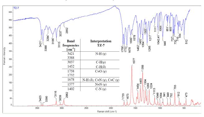
Figure 1. IR and Raman spectra of TZ-7.
