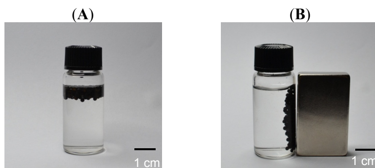
Figure 5. Iron oxide nanoparticle-loaded chitosan spheres were attracted to wall of the vial using an external magnetic field.
