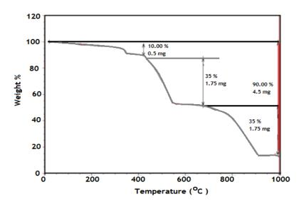
Figure 3. TGA thermogram of PAMPS-Na-co-St/magnetite composite.
