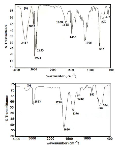
Figure 1. FTIR specta of (a) oleic acid coated magnetite and (b) PAMPS-Na-co-St/magnetite composite.
