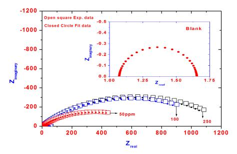
The impedance spectra exhibit one single capacitive loop, which indicates that the corrosion reaction is controlled by a charge transfer reaction. It is worth noting that the presence of inhibitor does not change the mechanism of steel dissolution [40]. It is evident that the impedance diagrams are not perfect semicircles, which is related to the frequency dispersion as a result of the roughness and inhomogeneity of the steel surface [41].
