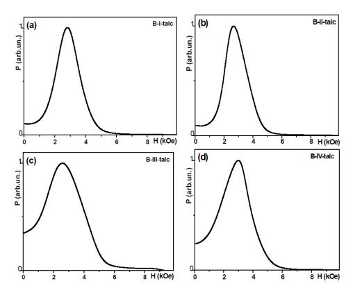
To understand rather large linewidths one can take into account work of Kale *et al.* [19] in which they have found that even in single crystal  $Fe_3O_4$  samples, the narrowest linewidths were of the order of 1 kOe, *i.e.*, rather high line widths is typical for ferrites.
