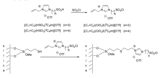
The presence of the unsaturated side chain made it possible to form a covalent bond with mercaptopropylated silica by a radical chain transfer reaction [11,30,31]. The disappearance of the characteristic peaks of S–H at 2565 cm<sup>-1</sup> and the allyl group at 1647 cm<sup>-1</sup> in the FT-IR spectra, as well as the lack of the carbon signals typical for an allyl group in the solid state <sup>13</sup>C-NMR proved the formation of the thioether bond [30].
