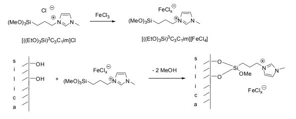
Scheme 4. Immobilisation of a Lewis acidic IL by a stepwise procedure.
