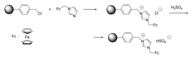
Scheme 14. Grafting of a ferrocenyl IL on Merrifield resin [63].
