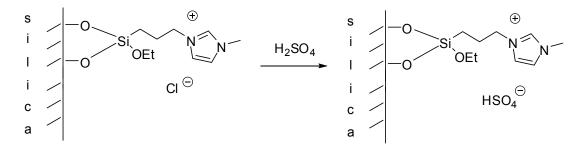
Scheme 10. Preparation of a SILP with a Brønsted acidic IL grafted on a silica support.
