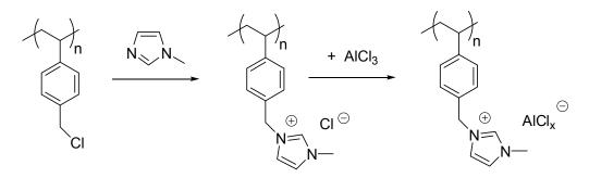
These catalysts were found to be stable to air and moisture retaining their activity for more than a year [32]. This stability was attributed to the hydrophobic nature of polystyrene that was able to protect the water-sensitive Lewis acid from hydrolysis by atmospheric moisture [34].
