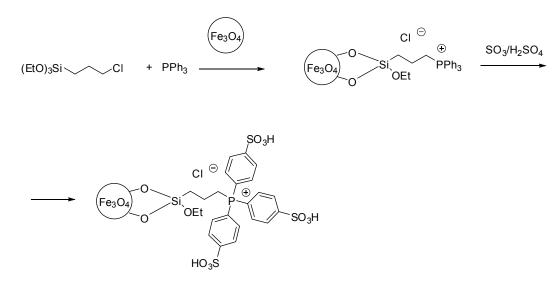
The advantages of magnetic nanoparticles was maintained after the grafting, the particle diameters of the nanoparticles remained in the range of 8–13 nm. As it could be expected, a slight decrease of the saturation magnetisation of the nanoparticles was observed that was due to the successful grafting of ionic liquids on the surface [59].
