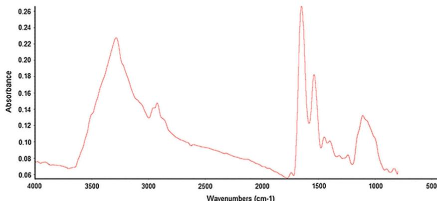
**Figure 1.** Representative mid-infrared (mid-IR) spectrum of yellow canola (*Brassica napus*) seed. Reproduced with permission from [25], published by Elsevier, 2014.
