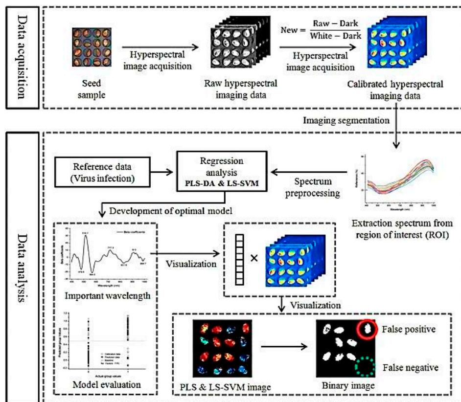
**Figure 4.** Flow work of hyperspectral imaging for detection of cucumber green mottle mosaic virus-infected watermelon seeds. Reproduced with permission from [57] published by Elsevier, 2016.
