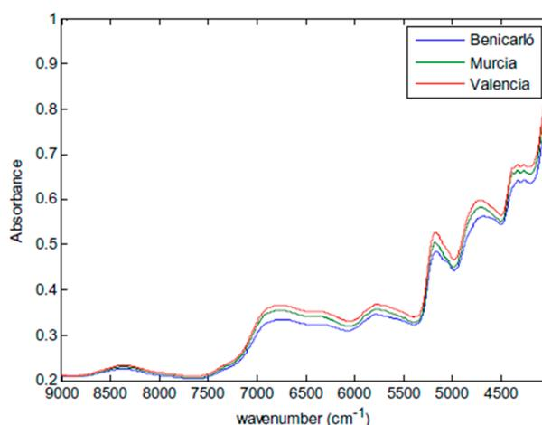
**Figure 2.** Mean near-IR spectra of artichoke samples from three different Spanish origins: Castellon (Alcachofa de Benicarló), Valencia and Murcia. Reproduced with permission from [32] published by Elsevier, 2016.
