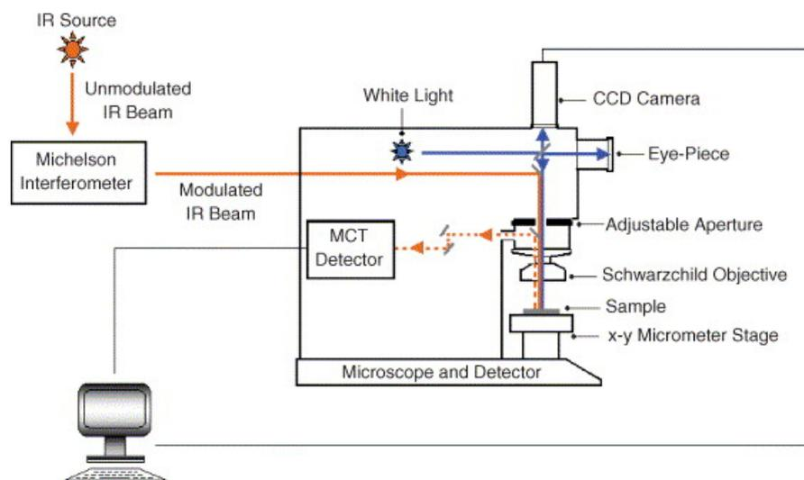
Figure 3. Block diagram of infrared imaging obtained from [44].
