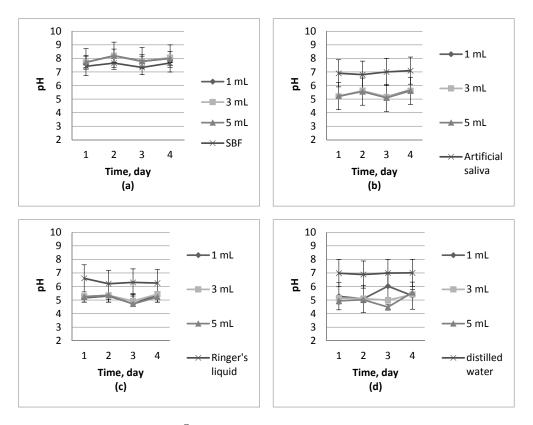
Figure 3. Incubation of Beetosan<sup>®</sup> hydrogels in: (a) SBF; (b) artificial saliva; (c) Ringer's liquid; and (d) distilled water.
