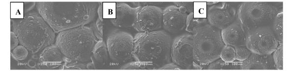
**Figure 8.** SEM microphotographs of Beetosan<sup>®</sup> hydrogels modified with: (**A**) 1 mL; (**B**) 3 mL; (**C**) 5 mL of nanosilver.
