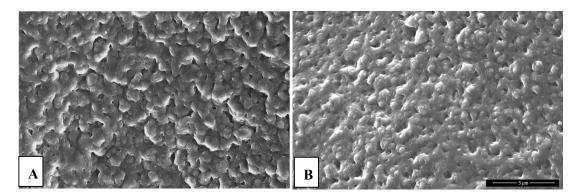
**Figure 7.** SEM microphotographs of chitosan hydrogels: (**A**) without additive; (**B**) modified with 5 mL silver nanoparticles.
