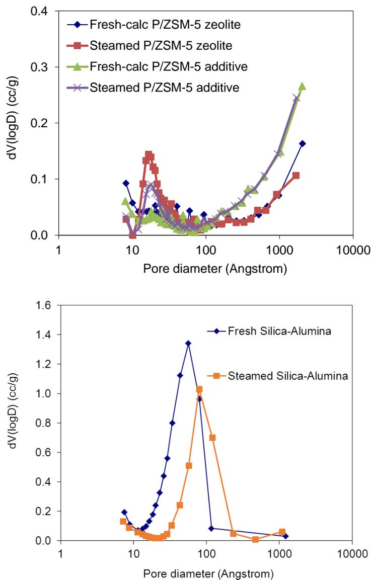
**Figure S3.** Pore size distribution curves based on the BJH analysis of the  $\text{N}_2$  adsorption data of fresh-calcined and steamed P/H-ZSM-5 pure zeolite, P/ZSM-5 additive and silica-alumina; steaming conditions were  $770^\circ\text{C}$ , 7 hrs, 50% steam/He.
