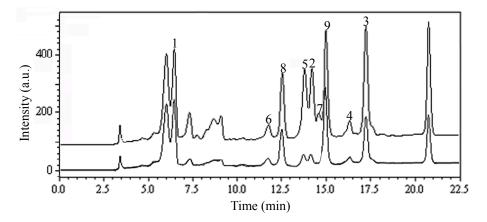
**Figure 2.** DPPH-HPLC chromatograms of *n*-butanol extract of *Lonicera japonica* leaves. Experimental conditions: Shim-pack VP-ODS column (250 mm × 4.6 mm, i.d., 5 µm); Column temperature: 25 °C; Flow rate: 1.0 mL/min; Detection: 254 nm; Injection volume: 10 µL. HPLC conditions are as follows: eluent A (MeOH) and eluent B (0.3% acetic acid in water, v/v), linear gradient combinations: at t = 0, 70% B; at t = 20 min, 40% B; at t = 22.5 min, 40% B. a.u.: arbitrary unit.
