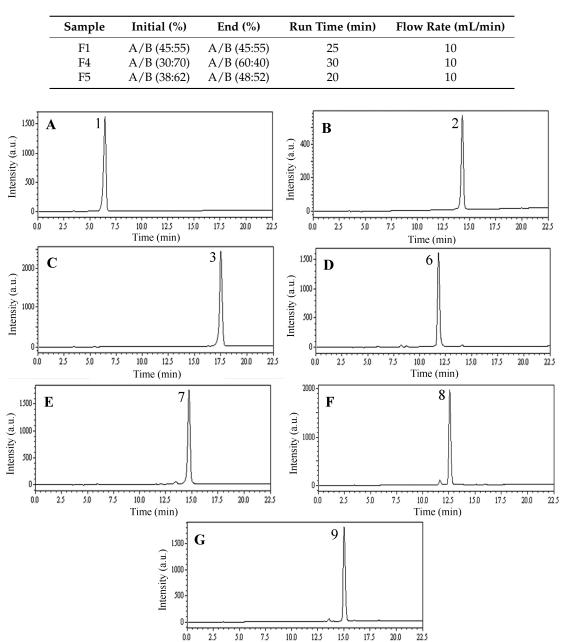
**Table 3.** Processing conditions for the preparative HPLC separations of sub-fractions F1, F4 and F5. (A: MeOH, B: 0.3% acetic acid in water, v/v).
