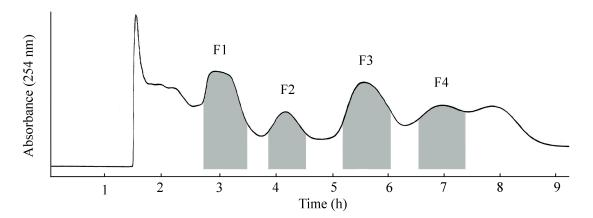
**Figure 3.** Chromatogram of the crude extract by HSCCC. Two-phase solvent system: methyl *tert*-butyl ether/*n*-butanol/acetonitrile/water (0.5% acetic acid) (2:2:1:5, *v/v*); Mobile phase: the lower phase; Flow rate: 2.0 mL/min; Revolution speed: 850 rpm; Detection wavelength: 254 nm; Sample size: 1.0 g; Injection volume: 10 mL; Retention of stationary phase: 47.3%; F2: rhoifolin; F3: luteoloside.
