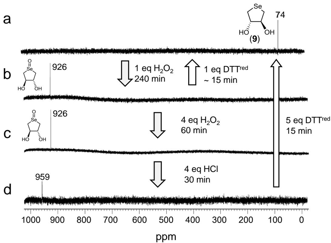
**Figure S5:**  $^{77}\text{Se}$  NMR spectral changes during redox reaction of **9** in  $\text{D}_2\text{O}$  at 298 K. Reaction conditions: **a**, Selenide **9** (0.024 mmol) in  $\text{D}_2\text{O}$  (500  $\mu\text{L}$ ). **b**, To **a** was added  $\text{H}_2\text{O}_2$  (0.024 mmol). **c**, To **b** was added  $\text{H}_2\text{O}_2$  (0.096 mmol). **d**, To **c** was added  $\text{HCl}$  (0.096 mmol).
