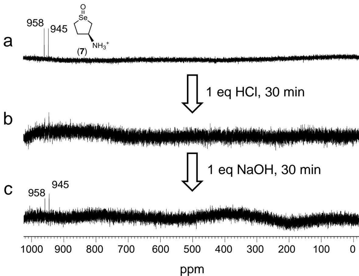
**Figure S4:**  $^{77}\text{Se}$  NMR spectral changes during acidification and neutralization of the selenoxide derived from selenide **7** in  $\text{D}_2\text{O}$  at 298 K. Reaction conditions: **a**, Selenide **7** (0.024 mmol) and  $\text{H}_2\text{O}_2$  (0.024 mmol) were mixed in  $\text{D}_2\text{O}$  (500  $\mu\text{L}$ ). **b**, To **a** was added HCl (0.024 mmol). **c**, To **b** was added NaOH (0.024 mmol).
