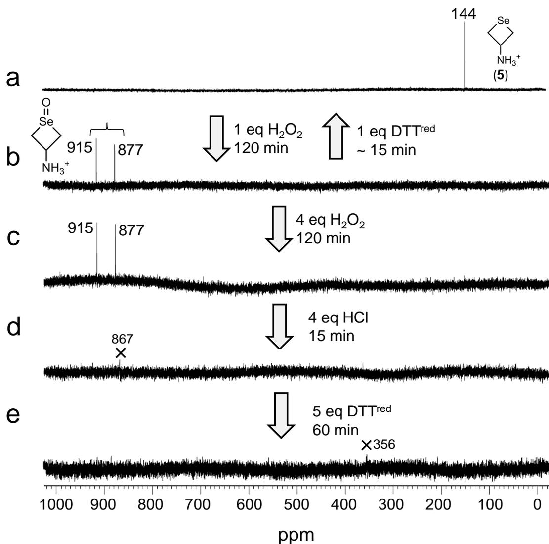
**Figure S2:**  $^{77}\text{Se}$  NMR spectral changes during the redox reactions of **5** in  $\text{D}_2\text{O}$  at 298 K. Reaction conditions: **a**, Selenide **5** (0.024 mmol) in  $\text{D}_2\text{O}$  (500  $\mu\text{L}$ ). **b**, To **a** was added  $\text{H}_2\text{O}_2$  (0.024 mmol). **c**, To **b** was added  $\text{H}_2\text{O}_2$  (0.096 mmol). **d**, To **c** was added  $\text{HCl}$  (0.096 mmol). **e**, To **d** was added  $\text{DTT}^{\text{red}}$  (0.12 mmol).
