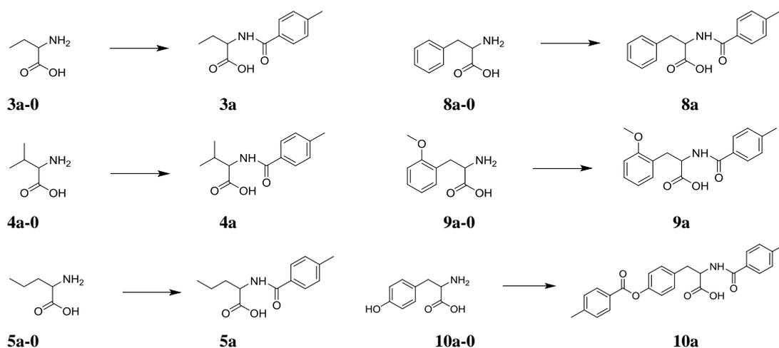
To a solution of amine (1.0 eq) in 15 ml 1N NaOH at 0 °C is added 4-Methylbenzoyl chloride dropwise (1.03 eq). The solution is stirred at rt for 2 hours until the reaction is complete based on TLC (PE:EA = 1:1). And then it is quenched with conc. HCl to pH = 2. The precipitate is filtered and the resulting residue is recrystallized in EtOAc/Hex to give the key intermediate as a white solid.
