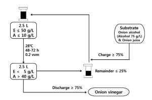
**Figure 7.** Schematic diagram of the semi-continuous fermentation process. E represents ethanol concentration and A represents acetic acid concentration.
