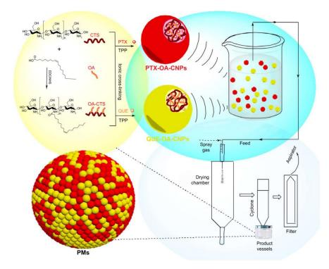
**Figure 1.** Synthesis and preparation scheme of PMs (PMs, polymeric microspheres; CTS, chitosan; OA, oleic acid; OA-CTS, OA-conjugated CTS; EDC, 1-(3-dimethylaminopropyl)-3-ethylcarbodiimide hydrochloride; NHS, *N*-hydroxysuccinimide; PTX, paclitaxel; TPP, sodium tripolyphosphate; QUE, quercetin; PTX-OA-CNPs, nanoparticles loaded with PTX; QUE-OACNPs, nanoparticles loaded with QUE); reproduced with the permission from [59], Copyright (2017) DOVE Medical Press.
