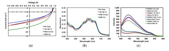
**Figure 8.** (a) JV curves for best devices; (b) thin film absorption profiles for 50:50 PBDB-T/1 blends; (c) thin film emission profiles for pure PBDB-T and 50:50 PBDB-T/1 blends. Plots are for devices as cast, TA at  $150 \degree$ C for 5 min, SVA from *o*-DCB for 15 min, and with a DPE 3% (*v*/*v*) additive.
