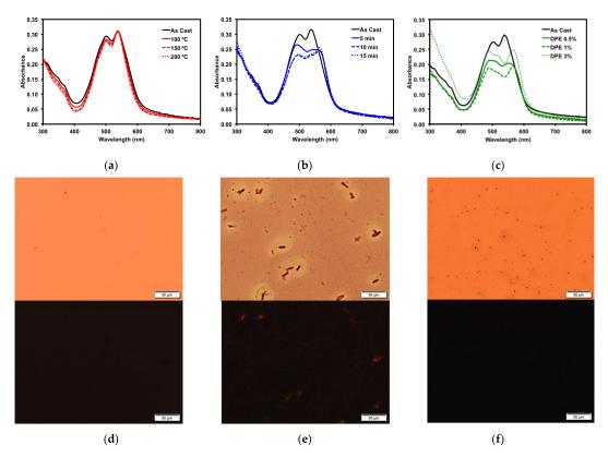
**Figure 5.** Optical absorption profiles of **1** with (**a**) thermal annealing; (**b**) *o*-DCB solvent vapour annealing; (**c**) DPE solvent additive. POM images of (**d**) 150 °C TA film; (**e**) 15 min *o*-DCB SVA film; and (**f**) 3% v/v DPE additive film under normal (top) and cross-polarized light (bottom). Images were taken at  $20 \times$  magnification.
