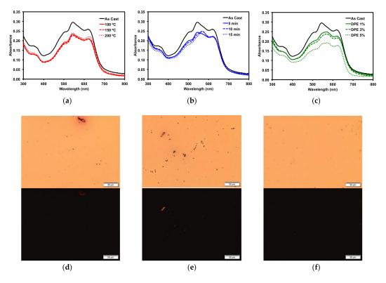
**Figure 6.** Absorption profiles of 50:50 PBDB-T/**1** blend with (**a**) TA; (**b**) *o*-DCB SVA; (**c**) DPE solvent additive. POM images of (**d**) 150 °C TA film; (**e**) 15 min *o*-DCB SVA film; and (**f**) 3% *v*/*v* DPE additive film under normal (top) and cross-polarized light (bottom). Images were taken at 20× magnification.
