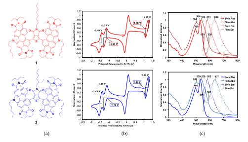
Figure 3. (a) Compounds 1 and 2; (b) cyclic voltammograms (with ferrocene internal standard) with onset potentials and  $E_{1/2}$  potentials shown; (c) solution and thin film absorption and emission profiles with  $\lambda_{max}$  and intercept between absorption and emission profiles,  $\lambda_{int}$ , shown. Emission spectra were recorded with excitation at 530 nm.
