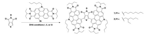
**Figure 2.** Reaction scheme for the synthesis of compounds **1** and **2**. (i) Toluene, 120 °C, Cs<sub>2</sub>CO<sub>3</sub>, pivalic acid, Pd(Herrmann-Beller), and P(*o*-anisyl)<sub>3</sub>; (ii) DMA, 80 °C, Cs<sub>2</sub>CO<sub>3</sub>, pivalic acid, and Silia*Cat*<sup>®</sup> DPP-Pd; and iii) toluene, 120 °C, Cs<sub>2</sub>CO<sub>3</sub>, pivalic acid, and Silia*Cat*<sup>®</sup> DPP-Pd.
