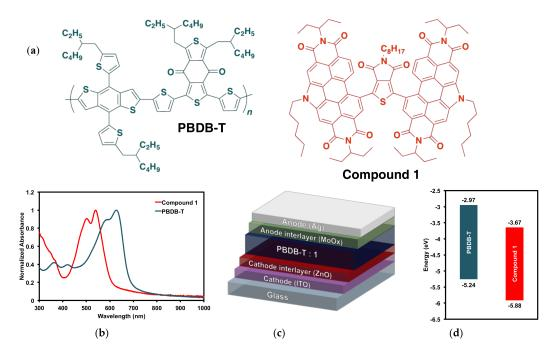
**Figure 7.** (**a**) PBDB-T donor polymer PBDB-T and (PDI)<sub>2</sub>octTPD (**1**) acceptor; (**b**) thin film absorption profiles; (**c**) device architecture; (**d**) electronic energy levels.
