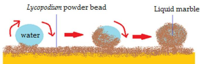
**Figure 1.** Obtaining liquid marbles by rolling water drops into a *Lycopodium* powder bed.
