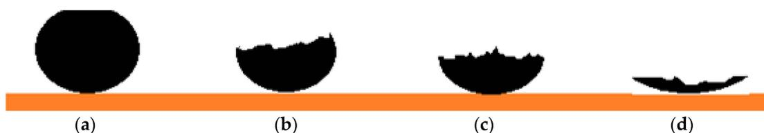
**Figure 9.** Plan and horizontal views of PTFE liquid marbles during evaporation: (a) initial liquid marble; (b) the marble begins to shrink as the shell wrinkles; (c) the outer shell is thickened and bulked; (d) liquid marble collapse.
