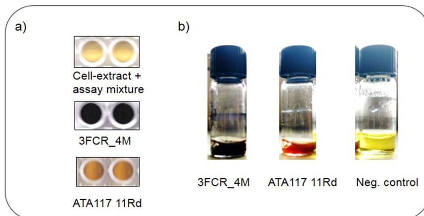
**Figure 1.** Screening for 3-converting  $\omega$ -TAs. (a) **4** was used as the amine donor in the screening. High activity resulted in dark precipitates. A yellow color indicates that no or low activity is present. For brown and orange colors it remains unclear whether enzyme activity is present. Cell extracts mixed with assay ingredients are displayed as negative control. (b) Result of 1 mL scale experiments after 24 h at 30 °C.
