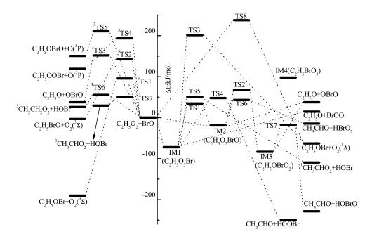
**Figure 2.** Energetic profiles of the  $C_2H_5O_2$  + BrO reaction at the QCISD(T)/6-311++G(2df,2p)//B3LYP/6-311++G(2df,2p) levels.
