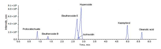
Figure 1. UPLC-MS chromatograms of 7 standard target compounds.
