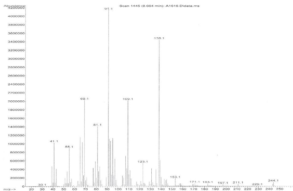
**Figure S3.** MS spectrum of (-)-isopulegol benzyl ether (**1**).
