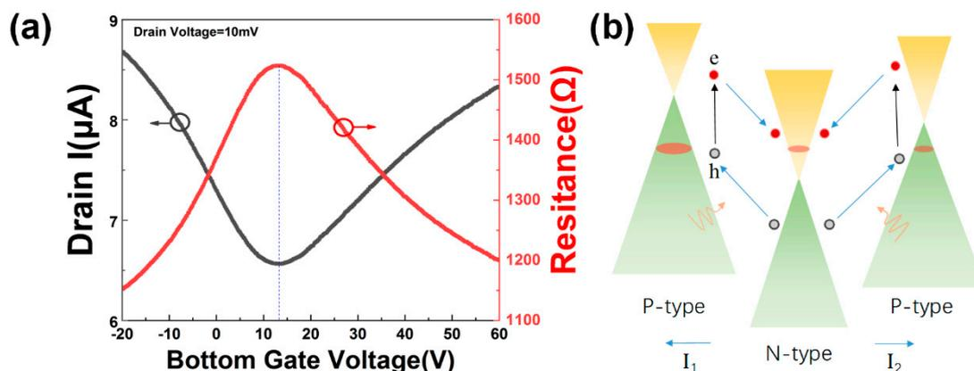
**Figure 4.** (a) Transfer characteristic curve of bottom gate graphene FET (field effect transistor) on Si/SiO<sub>2</sub> substrate. The monolayer graphene transferred on the Si/SiO<sub>2</sub> exhibits p-type. (b) Band structure of the horizontal p-n-p junction, blue arrows describe the movement of photo-induced electrons (red balls) and holes (gray balls).
