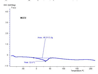
Differential Scanning Analysis (DSC) of Pure o-PDA
