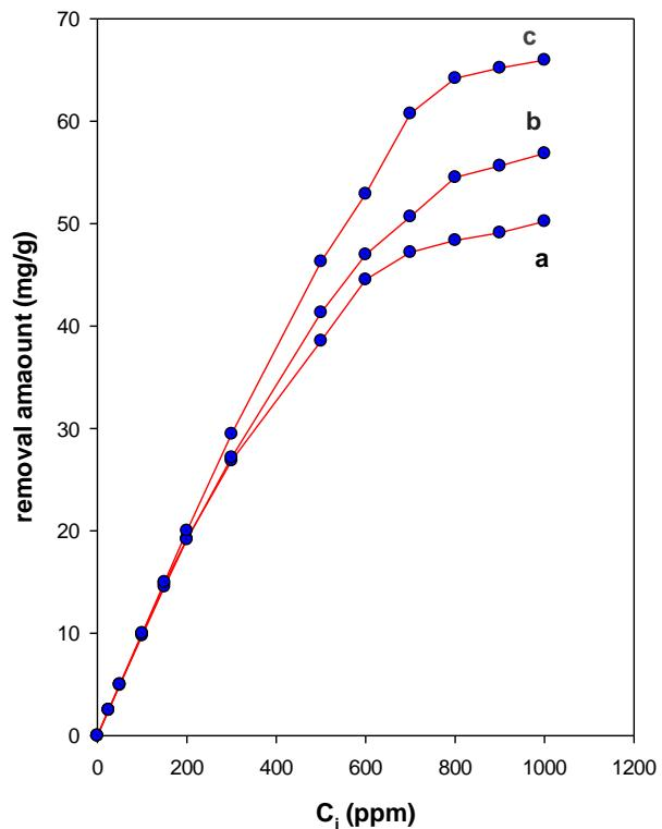
**Supplementary material 5.** Eosin removal properties of C16Cl-CN at different temperatures
