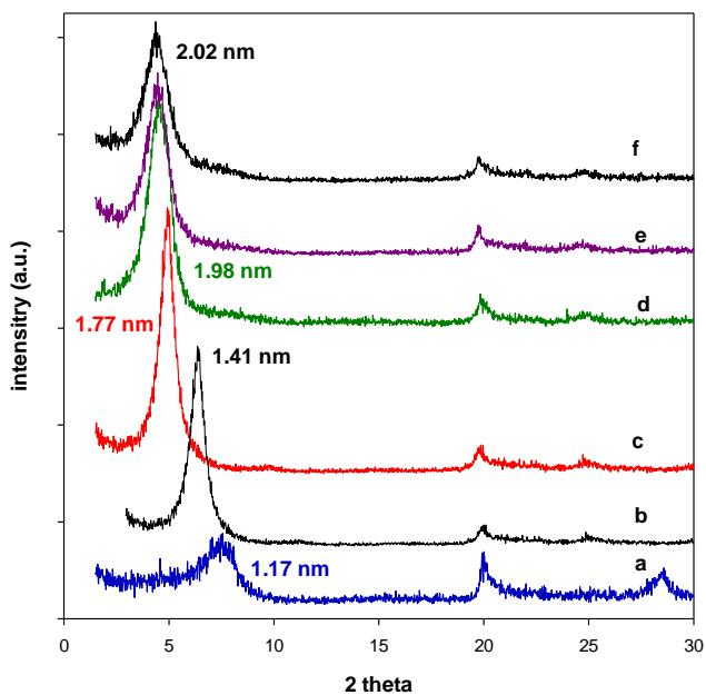
**Supplementary material 1.** Powder XRD patterns of (a) cloisite clay exchanged with C16Cl solution using different concentrations (b) 0.20 mM, (c) 0.40 mM; (d) 1.20 mM, (e) 1.60 mM, and (f) 3.20 mM.
