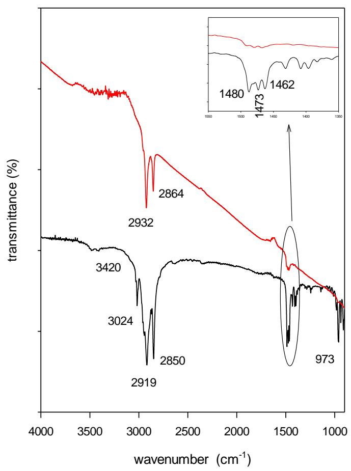
**Supplementary material 2.** FTIR spectra of solid C16TMABr salt (black) and liquid C16TMABr (red)
