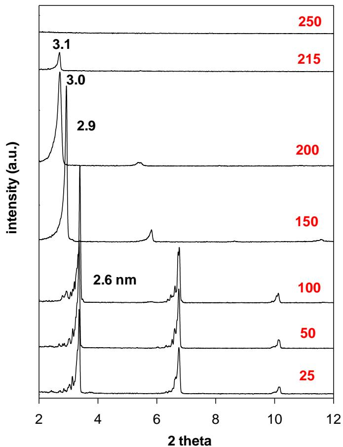
**Supplementary material 3.** *in-situ* Powder XRD patterns of C16TMABr salt preheated at different temperatures (°C).
