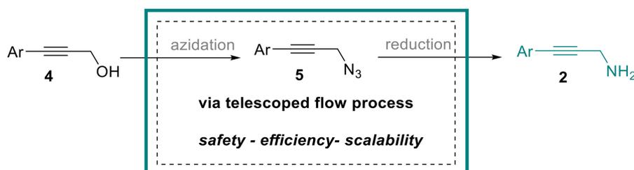
**Scheme 2.** Telescoped flow approach to propargylic amines **2**.
