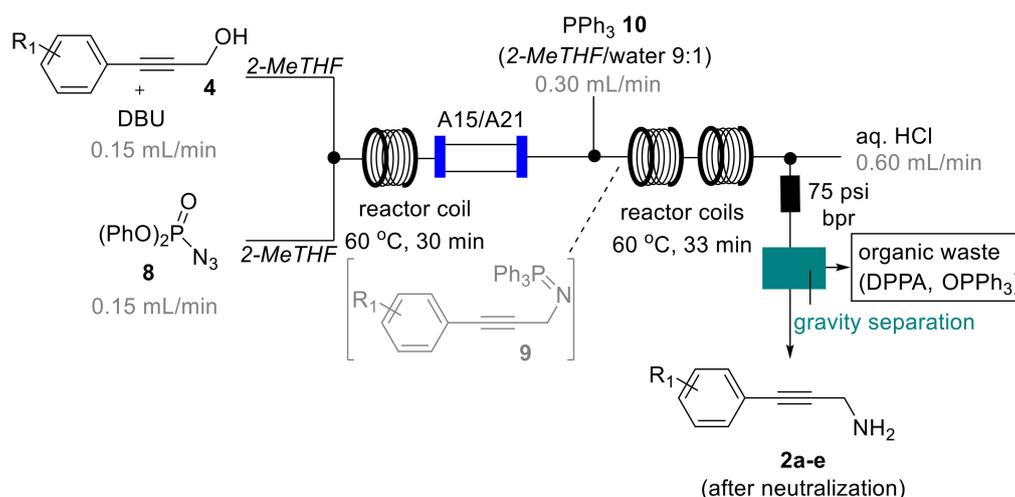
**Scheme 6.** Final telescoped flow process using 2-MeTHF.
