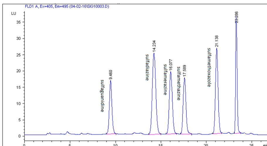
Figure 4. Chromatogram of feed sample spiked with five SAs at a concentration of 200  $\mu\text{g}/\text{kg}$  on a Zorbax Eclipse XDB C18 column with a mobile phase of 0.08% acetic acid in Milli-Q water/acetonitrile/methanol.
