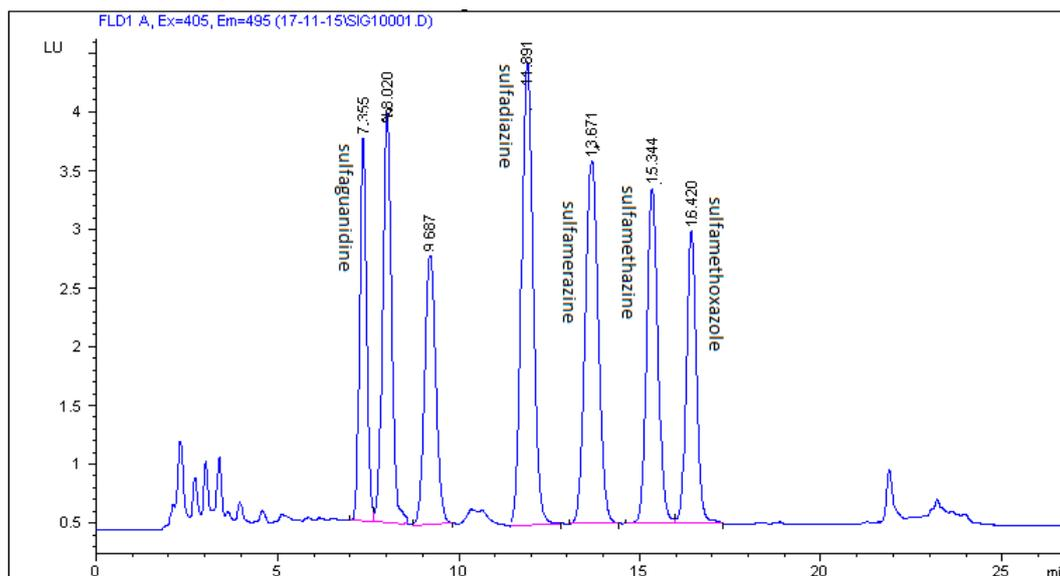
**Figure 6.** Chromatogram of feed sample spiked with five SAs at a concentration of 200  $\mu\text{g}/\text{kg}$  on a Zorbax Eclipse XDB C18 column with a mobile phase of 0.1% formic acid in Milli-Q water/acetonitrile/methanol.
