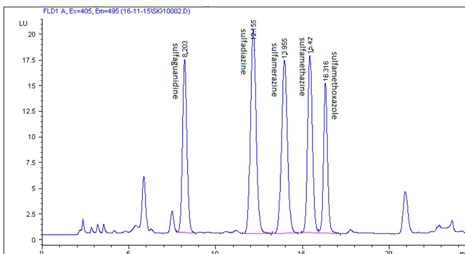
Figure 5. Chromatogram of feed sample spiked with five SAs at a concentration of 200  $\mu\text{g}/\text{kg}$  on a Zorbax Eclipse XDB C18 column with a mobile phase of 0.1% acetic acid in Milli-Q water/acetonitrile/methanol.
