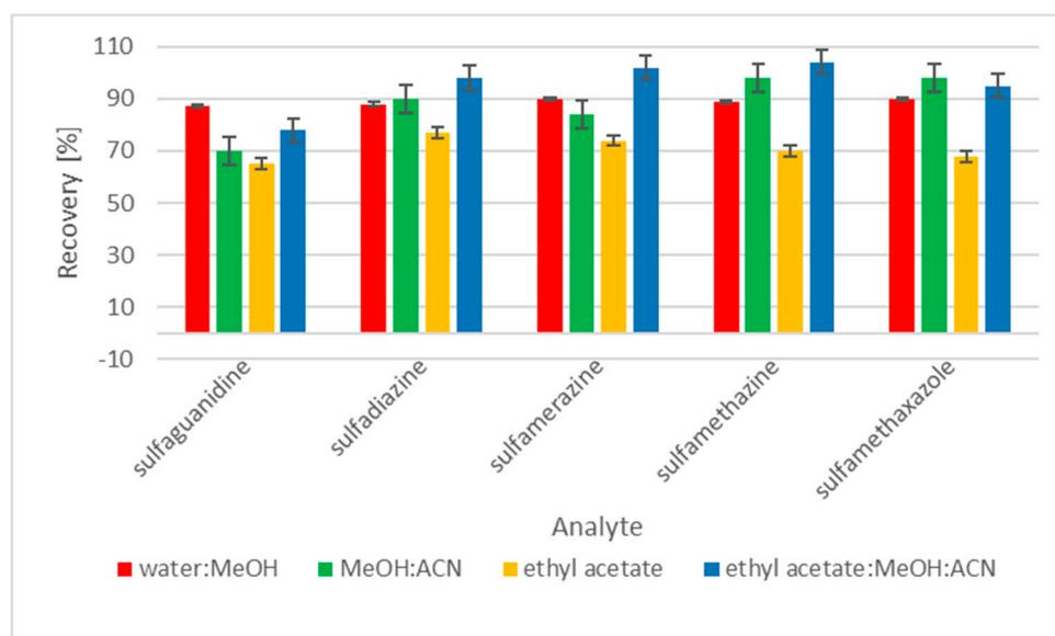
**Figure 1.** Recovery of sulfonamides employing different extraction solvents ( $n = 6$ ).
