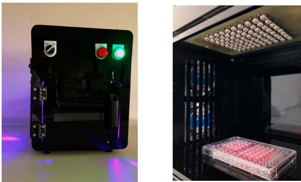
**Figure 5.** Photograph of the illumination device (left) and the 10 × 8 blue LED array (right).
