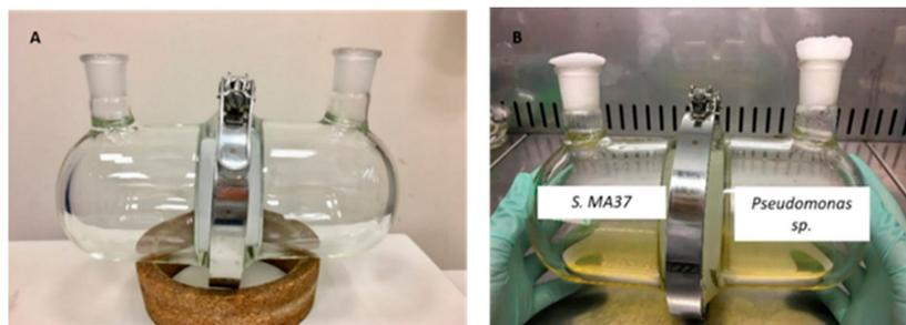
**Figure 1.** (A). Assembled co-culture device enabling separation of two independent cultures with a 0.22  $\mu\text{m}$  membrane filter and joined by a holding clamp. (B). Co-culture of *Streptomyces* sp. MA37 and *Pseudomonas* sp. prior to incubation.
