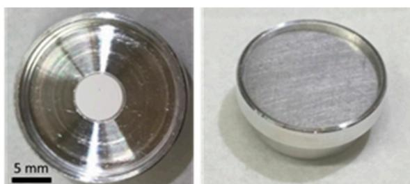
**Figure 2.** Pressed  $\text{CaO}$  target (6 mm  $\times$  0.5 mm) nestled in the indentation of an Al (99.5% pure) capsule. The capsule was sealed and prepared for irradiation at PSI's IP2 irradiation station.
