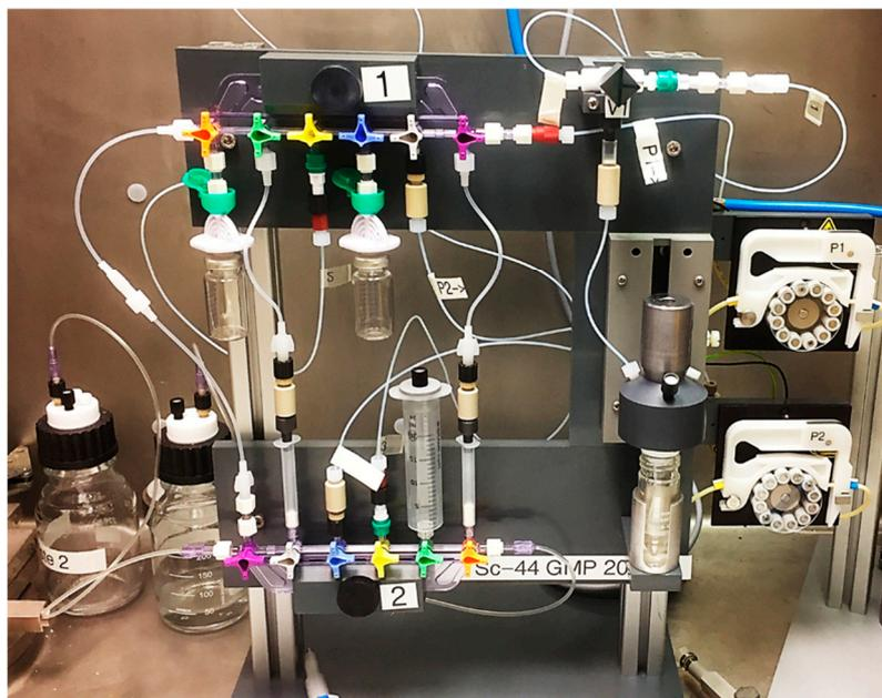
**Figure 6.** Schematic representation of the  $^{44}\text{Sc}$  chemical separation system (above), with the actual system—using disposable medical grade components—shown below. S1, S2, S3 in the scheme indicate the outside syringe lines (containing Bbraun non-return valves) to introduce the solutions used to perform the separation.
