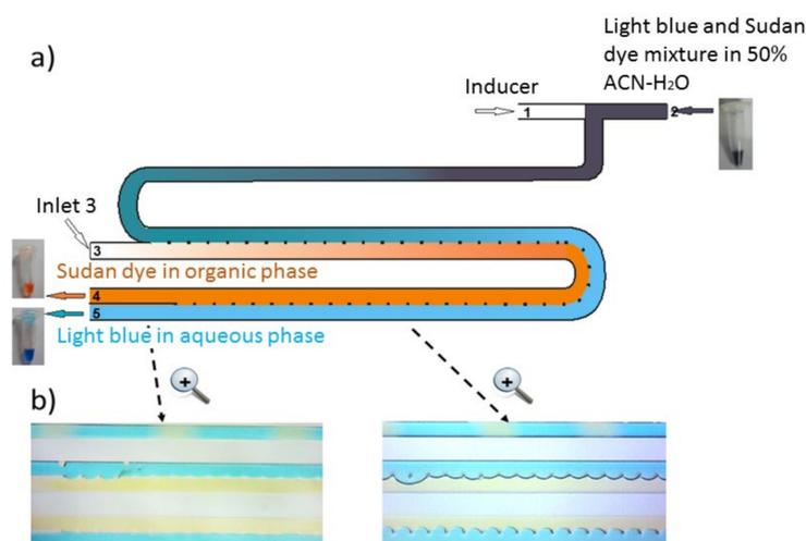
**Figure 1.** Schematic representation of the induced phase separation extraction chip: (a) lay-out of the IPSE chip when filled with a dye mixture (Indigo blue and Sudan red); (b) photos of parts of the IPSE chip while separating a blue-orange dye mixture by using the mixed inducer (dichloromethane–butyl acetate (2:8)).
