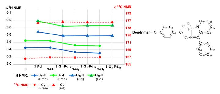
**Figure 12.** <sup>1</sup>H NMR data for the hydrogen atoms on the carbon adjacent to the nitrogen atom of both pyridine rings ( $C_{12}$ -H and  $C_{17}$ -H), and <sup>13</sup>C NMR data of the carbon of the imine bond ( $C_7$ ), for monomer and dendrimers, free and complexed in both cases.
