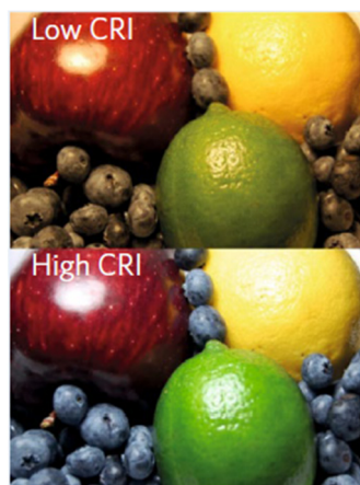
Figure 2. Difference in colour-rendering capabilities between high and low CRI. Reprinted with permission from Ref. [6]. 2017, Springer Nature: Nature Energy.
