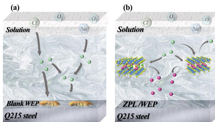
**Figure 9.** Anti-corrosion mechanism of (a) blank WEP and (b) ZPL/WEP.
