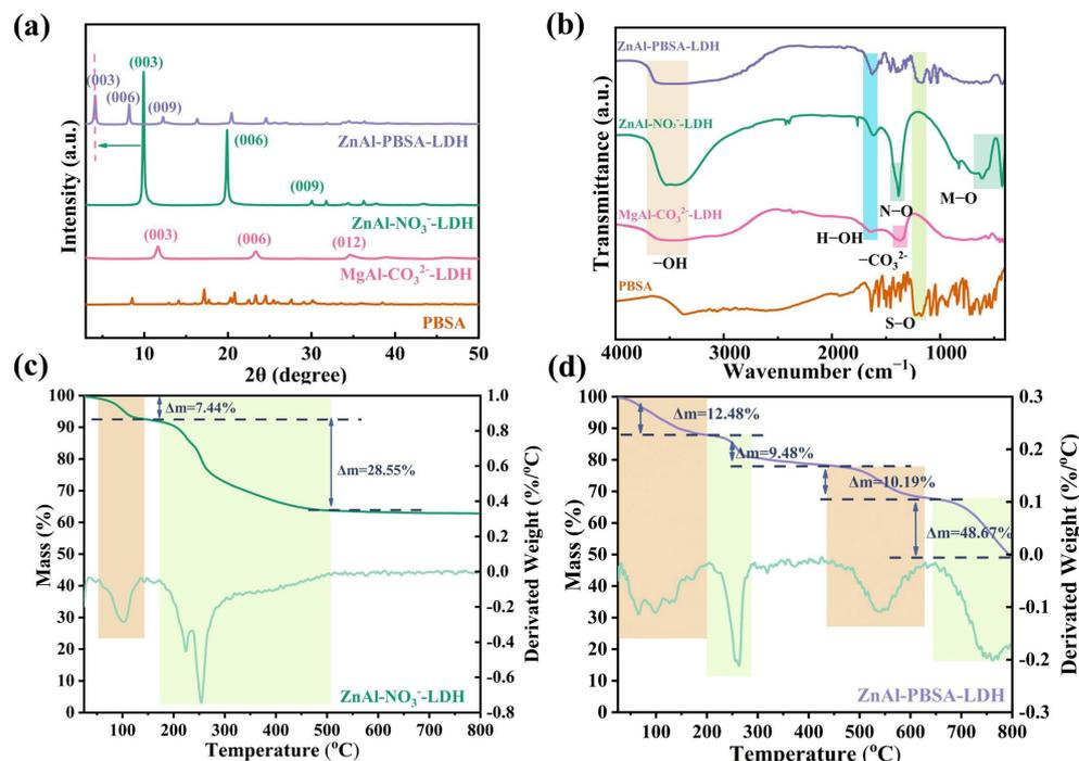
**Figure 2.** (a) XRD curves; (b) FTIR curves; TG-DTG curves of (c)  $\text{ZnAl-NO}_3^-$ -LDH and (d)  $\text{ZnAl-PBSA-LDH}$ .
