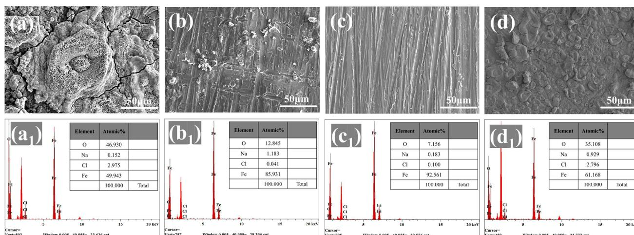
**Figure 8.** SEM images and EDS mapping of substrates coated by (a,a<sub>1</sub>) blank WEP, (b,b<sub>1</sub>) 4-ZPL/WEP, (c,c<sub>1</sub>) 6-ZPL/WEP, and (d,d<sub>1</sub>) 8-ZPL/WEP coatings after immersion of 30 days.
