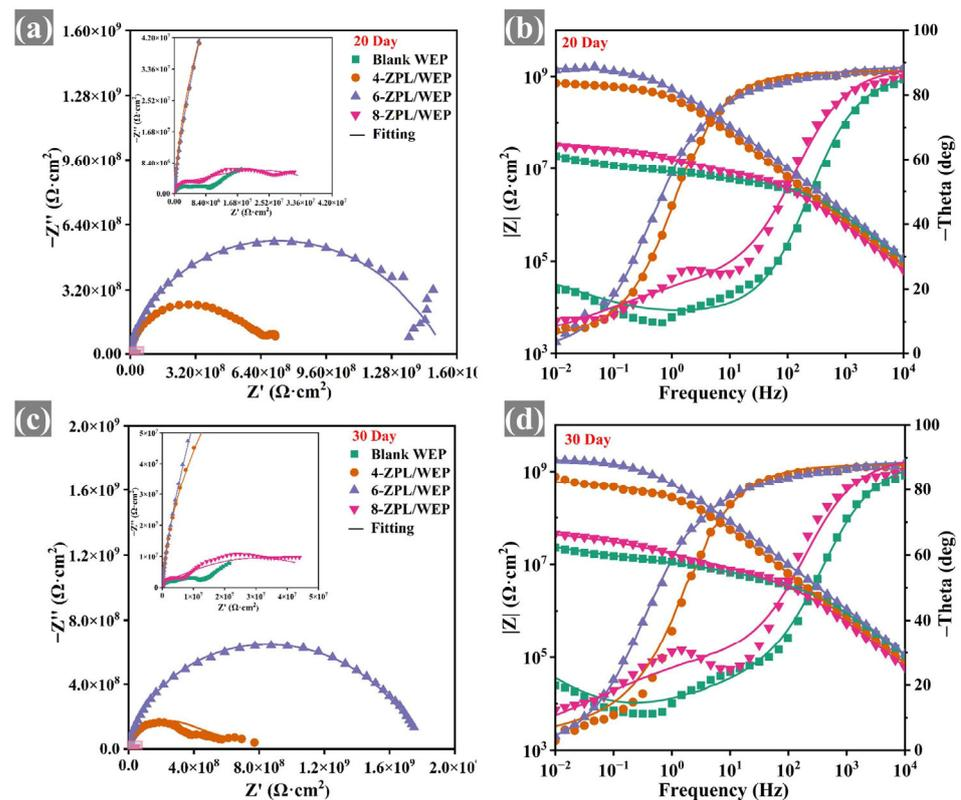
**Figure 6.** (a,c) Nyquist and (b,d) Bode plots of coated samples after 30 days immersion.
