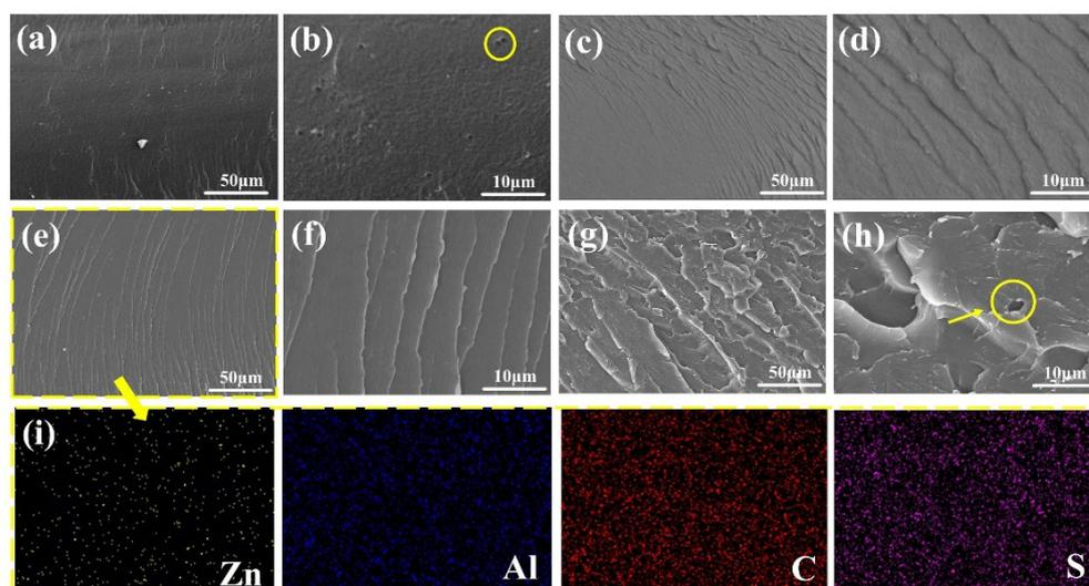
**Figure 3.** SEM images of the fractured surface of (a,b) blank WEP, (c,d) 4-ZPL/WEP, (e,f) 6-ZPL/WEP, and (g,h) 8-ZPL/WEP. The EDS mapping of (i) 6-ZPL/WEP.
