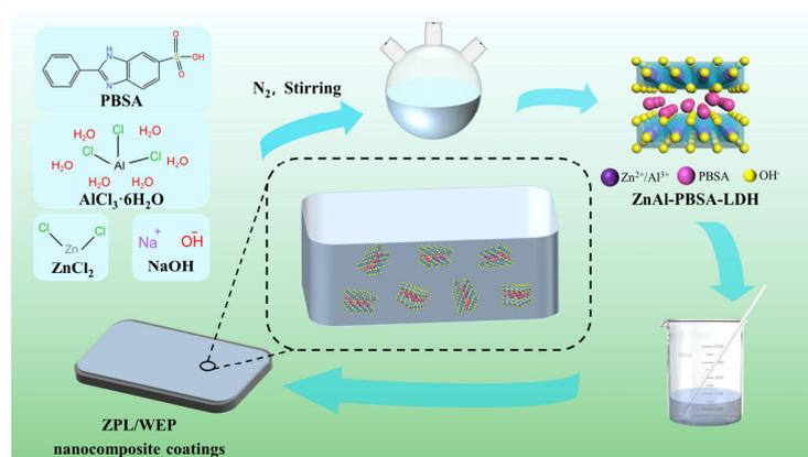
**Figure 10.** Schematic diagram of the synthesis and preparation of the LDH coating.
