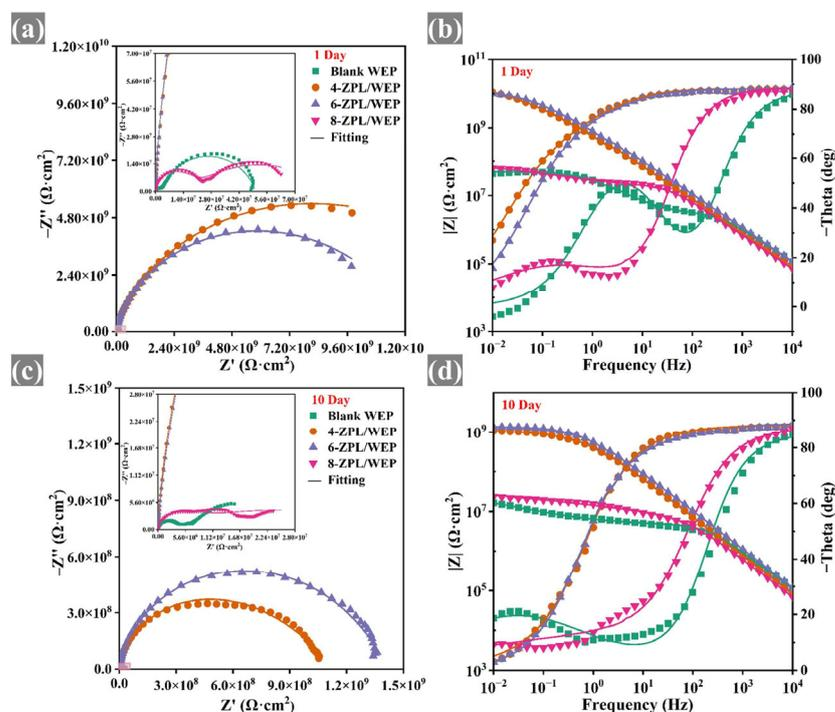
Figure 5. (a,c) Nyquist and (b,d) Bode plots of coated samples after 10 days immersion.
