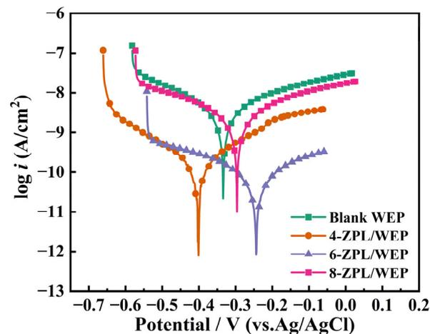
**Figure 7.** Potentiodynamic polarization curves of all coatings after 30 days of immersion in 3.5 wt.% NaCl solution.
