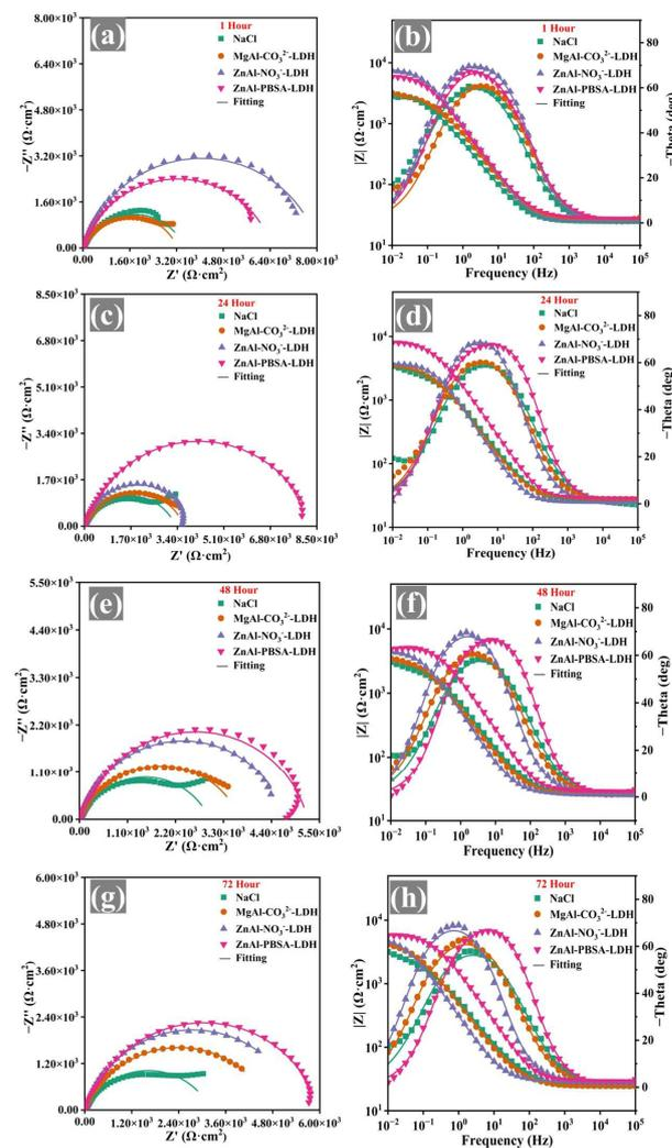
**Figure 4.** Nyquist plots and Bode-phase plots of the immersed bare steel samples in the blank solution and the extracted solutions of NaCl, MgAl-CO<sub>3</sub><sup>2-</sup>-LDH, ZnAl-NO<sub>3</sub><sup>-</sup>-LDH, and ZnAl-PBSA-LDH for (a,b) 1 h, (c,d) 24 h, (e,f) 48 h, and (g,h) 72 h.
