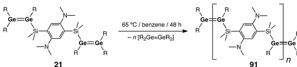
**Scheme 44.** The acyclic diene metathesis (ADMET) polymerization of *p*-phenylene-bridged tetragermadiene precursor **21** forming ADMET-poly(digermene) **91**.
