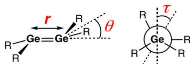
**Figure 3.** Structural parameters of digermenes (and other multiply bonded organogermanium compounds): bond length,  $r_{\text{Ge}=\text{Ge}}$ ; bent angle  $\theta$ ; and twist angle  $\tau$ .
