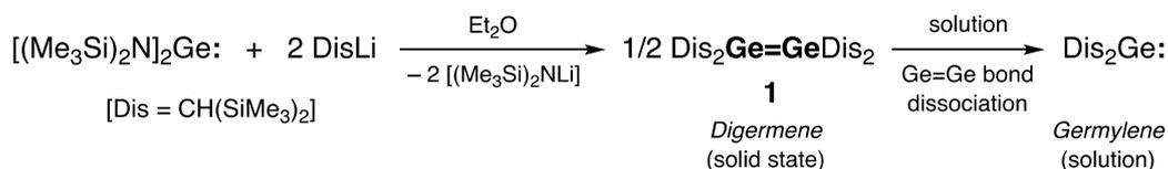
**Scheme 1.** Synthesis of the first isolable digermene  $\text{Dis}_2\text{Ge}=\text{GeDis}_2$  **1**.
