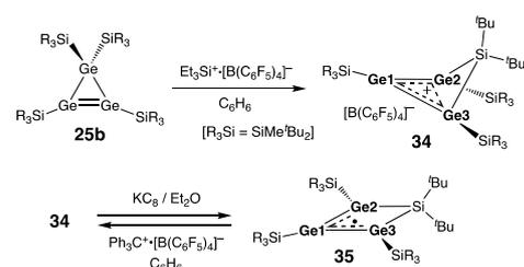
**Scheme 16.** Synthesis of silatri(germa)cyclobutenylium ion derivative **34**.
