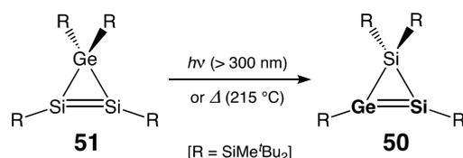
**Scheme 26.** Synthesis of the first isolable silagermene **50**.
