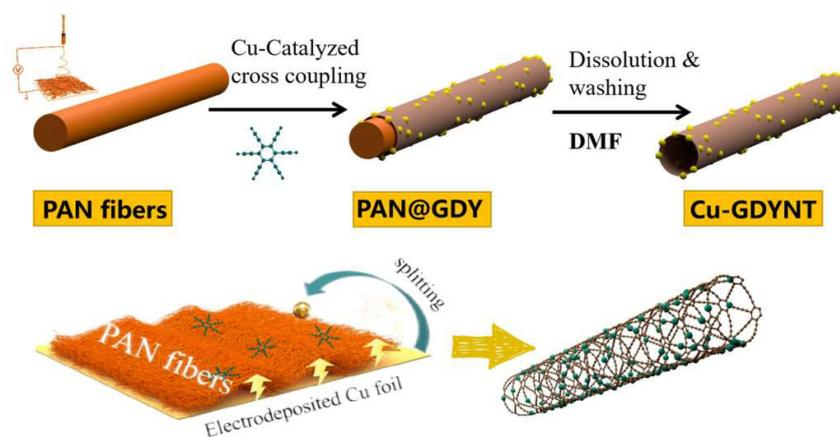
**Figure 1.** The fabrication process of the Cu-GDYNT.
