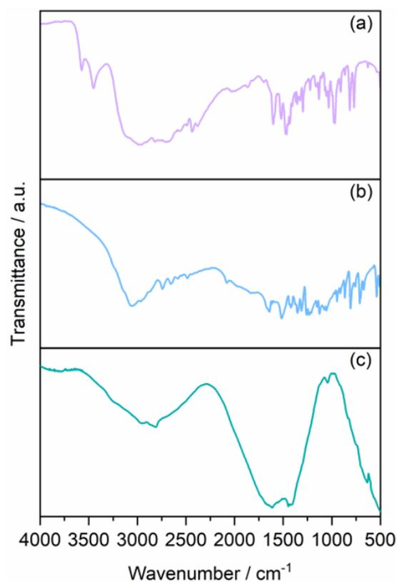
**Figure 6.** IR spectra of (a) trien, (b) L-glutamic acid, and (c) GQDs as solids onto silicon windows.
