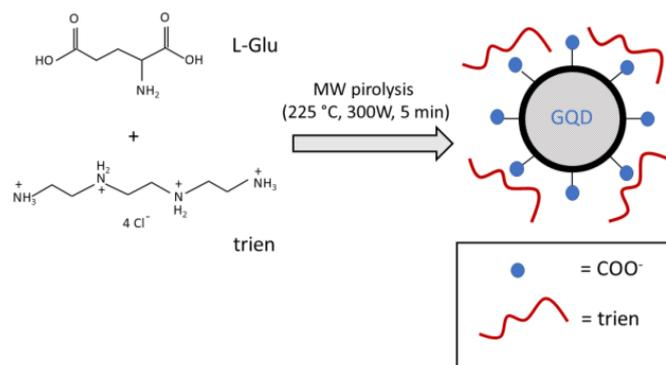
**Scheme 1.** Sketch diagram of the MW-assisted synthesis of GQDs used in this study.
