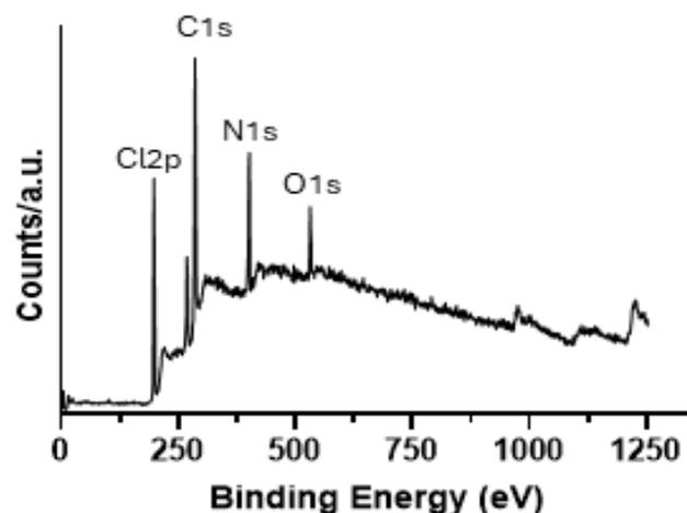
**Figure 3.** XPS survey spectrum for a blank mixture containing the precursors before the pyrolysis procedure.
