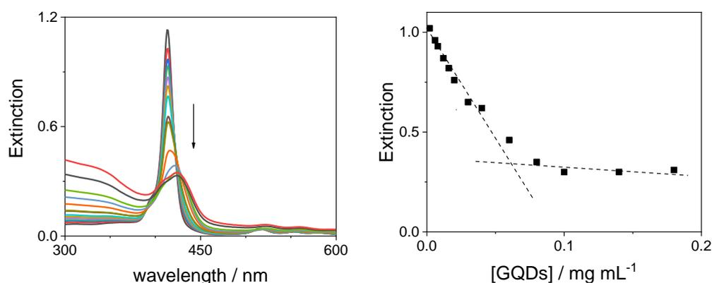
**Figure 7.** UV/Vis extinction spectral changes (left panel) and extinction at 413 nm (right panel) during the titration of TPPS<sub>4</sub><sup>4-</sup> with GQDs at neutral pH (the arrow marks the increasing GQD concentration). The dashed lines are a visual reference. Experimental conditions: [TPPS<sub>4</sub><sup>4-</sup>] = 3  $\mu$ M; [GQDs] = 0–0.18 mg/mL; phosphate buffer 1 mM, pH = 7; T = 298 K; cell path length 1 cm.
