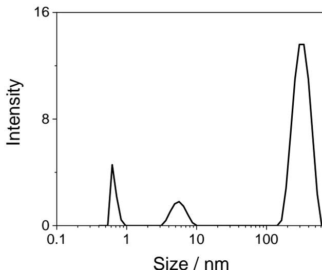
**Figure 2.** Distribution of particle size measured on an aqueous solution of GQDs (0.14 mg/mL) through the dynamic light scattering technique.
