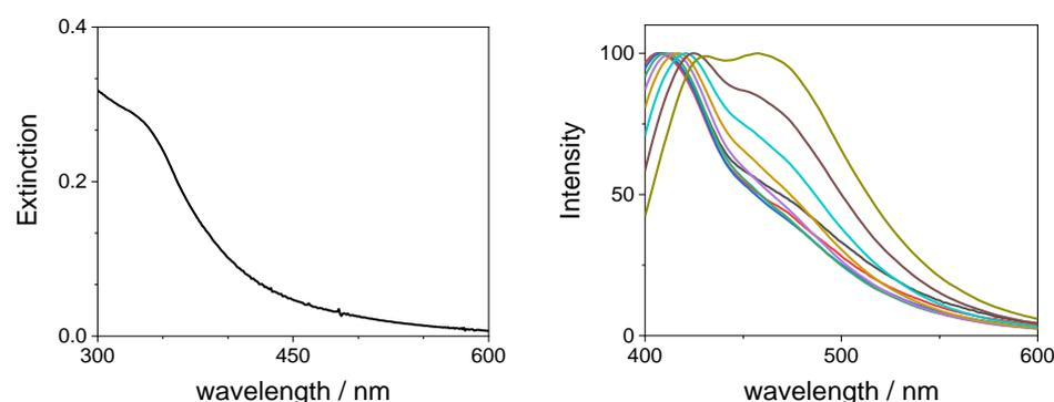
**Figure 1.** Spectroscopic features of an aqueous solution of GQDs (0.14 mg/mL): UV/Vis absorbance spectrum (left panel) and normalized fluorescence spectra (right panel, excitation wavelength from 310 to 390 nm).
