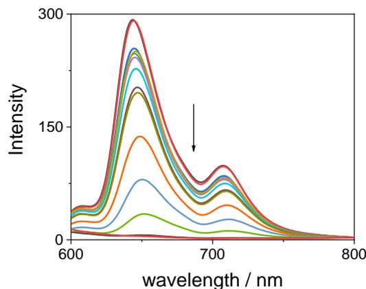
**Figure 8.** Fluorescence emission spectral changes during the titration of TPPS<sub>4</sub><sup>4-</sup> with GQDs at neutral pH (the arrow marks the increasing GQD concentration). Experimental conditions: [TPPS<sub>4</sub><sup>4-</sup>] = 3 μM; [GQDs] = 0–0.18 mg/mL; phosphate buffer 1 mM, pH = 7; T = 298 K; cell path length 1 cm; excitation wavelength 420 nm (isosbestic point in the UV/Vis titration).
