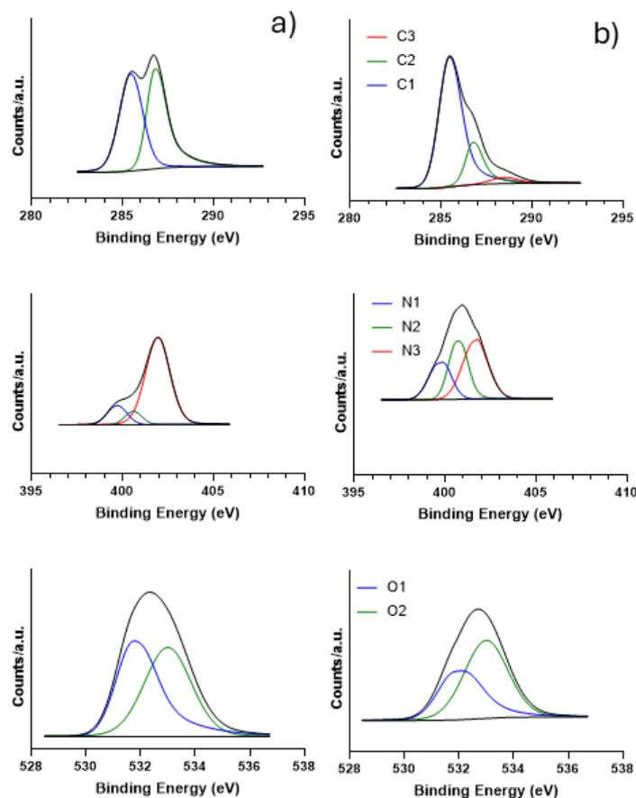
**Figure 4.** XPS spectra for the C1s, N1s, and O1s regions for (a) the sample before pyrolysis and (b) for GQDs.
