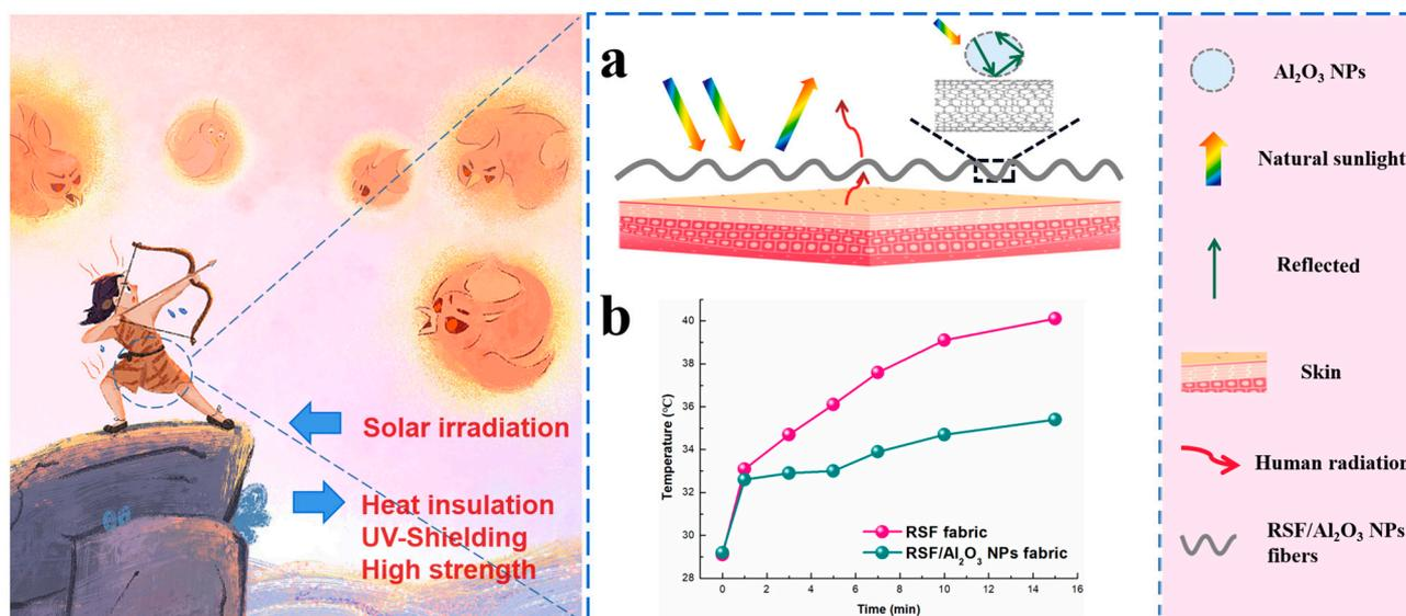
**Figure 1.** Schematic illustration of RSF/ $\text{Al}_2\text{O}_3$  NPs hybrid fibers with heat insulation and UV resistance. (a) Diagram of the photothermal conversion process with RSF/ $\text{Al}_2\text{O}_3$  NPs fabric. (b) Temperature change of RSF fabric and RSF/ $\text{Al}_2\text{O}_3$  NPs fabric under natural sunlight for 15 min.
