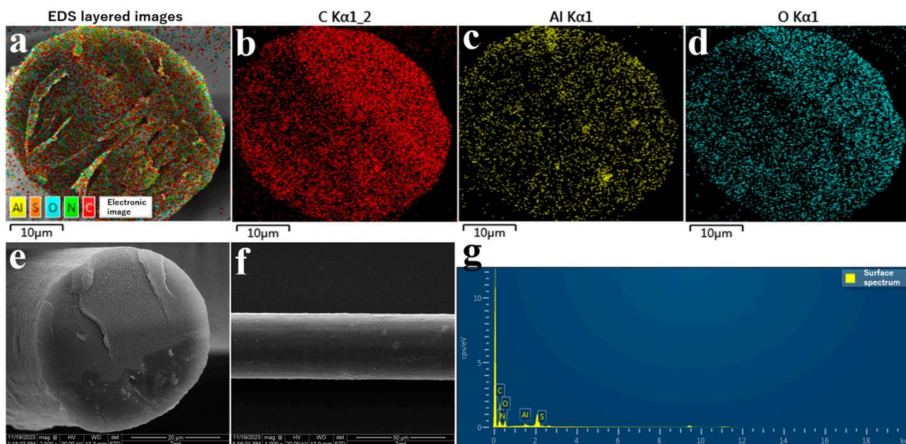
**Figure 2.** EDS images of 0.8 wt% RSF/ $\text{Al}_2\text{O}_3$  NPs hybrid fibers (a–d,g); SEM images of 0.8 wt% RSF/ $\text{Al}_2\text{O}_3$  NPs hybrid fibers (e) Internal structure; (f) Surface structure.
