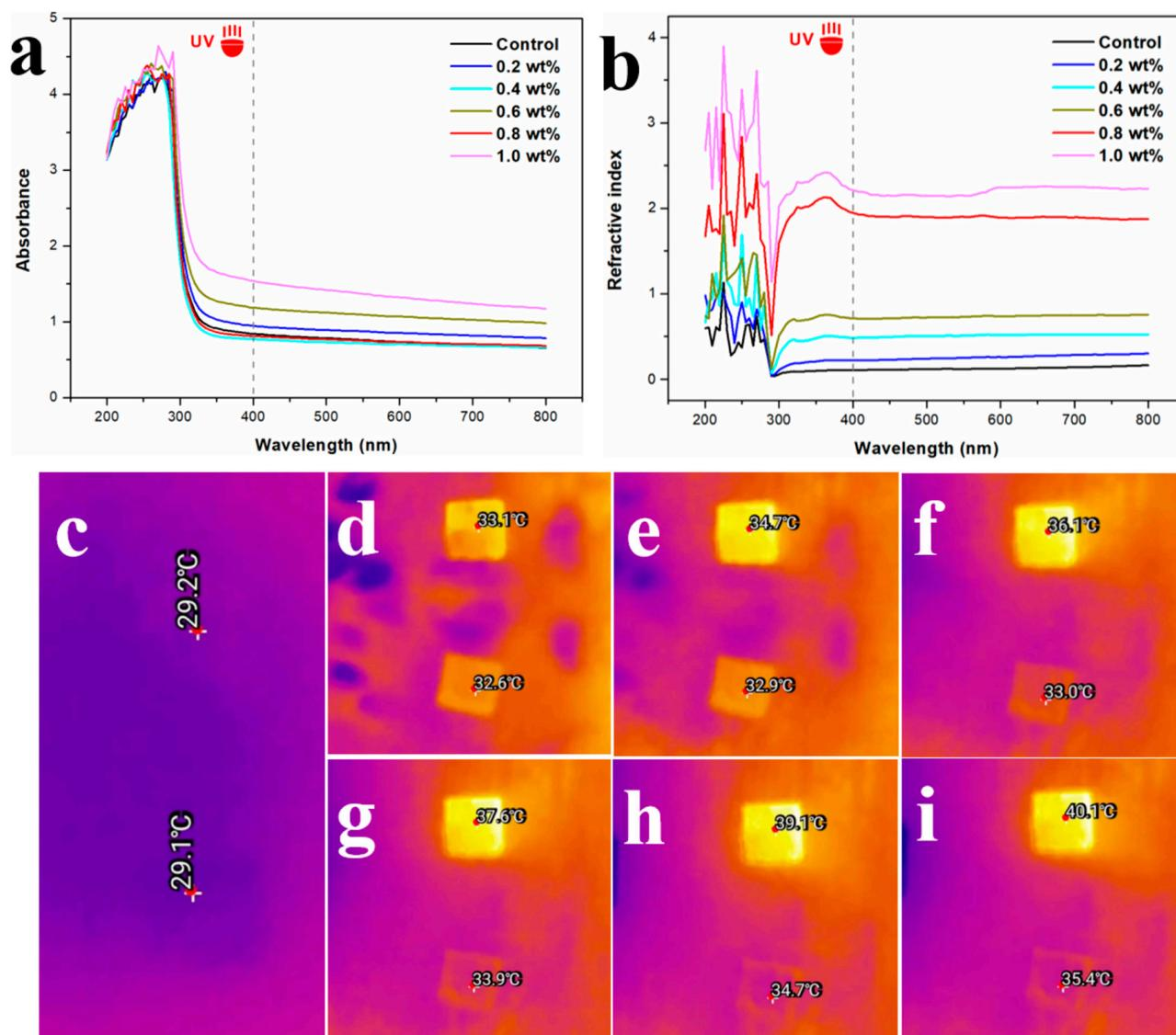
**Figure 4.** (a,b) UV absorption and refraction of RSF and RSF/ $\text{Al}_2\text{O}_3$  NPs hybrid fibers with different concentrations. (c–i) Initial thermal imaging picture and thermal imaging temperature picture of 0.8 wt% RSF/ $\text{Al}_2\text{O}_3$  NPs hybrid fibers in sunlight ((d–i) were real-time thermal imaging pictures when the illumination time is 1, 3, 5, 7, 10, 15 min, respectively).
