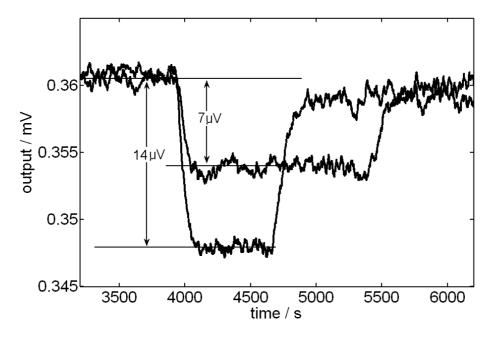
To be able to evaluate this effect, the calorimetric signal has been deconvolutioned by applying a derivative filter with a time constant  $\tau(t)$  which varies linearly during the injection interval, from 230 to 260 s, and an integrating filter with  $\tau^*=40$  s [19,22].
