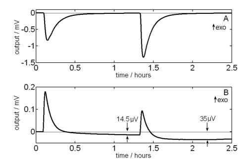
**Figure 4.** Energy of the second injection pulse corresponding to the Figure 3B (formamide + ethanediol). (a) Comparison among voltage values obtained from the ITC-curve and (b) from the deconvolutioned signal.
