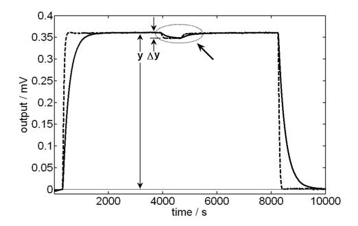
**Figure 2.** Injection effect during an electrical dissipation (see Figure 1). Extension of the deconvoluted signal in the injection interval for two different injection flows: 1  $\mu$ L/s ( $\Delta y$ =7  $\mu$ V) and 2  $\mu$ L/s ( $\Delta y$  = 14  $\mu$ V).
