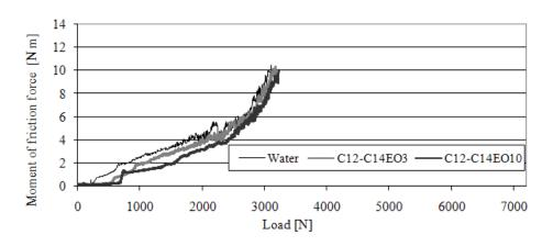
In the initial phase of the test the moment of friction force increases slightly until load takes the value of scuffing load ( $P_t$ ). Above that point,  $M_T$  increases sharply up to 10 N m, and load takes the value of seizure load ( $P_{oz}$ ). Compared to micellar solutions, there is a characteristic low, practically
