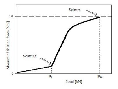
**Figure 6.** The course of changes in moment of friction force ( $M_T$ ) as a function of load (P) for water and 50% solutions of alcohols ethoxylated with 3 and 10 moles of ethylene oxide ( $C_{12}$ - $C_{14}$  EO<sub>3</sub> and  $C_{12}$ - $C_{14}$  EO<sub>10</sub>). Four-ball tester, rotational speed of spindle 500 rpm.
