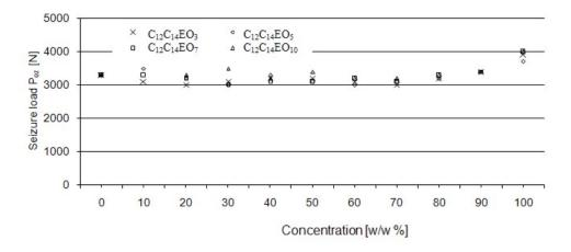
**Figure 9.** The effect of concentration on the value of limiting pressure of seizure ( $p_{oz}$ ) of aqueous solutions of alcohols ethoxylated with 3–C<sub>12</sub>-C<sub>14</sub> EO<sub>3</sub>, 5–C<sub>12</sub>-C<sub>14</sub> EO<sub>5</sub>, 7–C<sub>12</sub>-C<sub>14</sub> EO<sub>7</sub>, 10–C<sub>12</sub>-C<sub>14</sub> EO<sub>10</sub> moles of ethylene oxide. Four-ball tester, rotational speed of spindle 200 rpm, load increasing rate 409 N/s.
