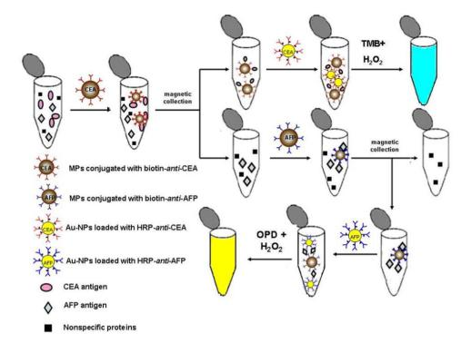
**Figure 2.** Colorimetric detection of CEA and AFP antigens. Only in the presence of antigens which are cognate with the antibodies loaded on the surfaces of MPs and Au-NPs, can the immunocomplexes be formed, and the characteristic blue and yellow colors of catalytic products be observed. Reprinted with permission from Ref. [45]. Copyright 2009 Elsevier.
